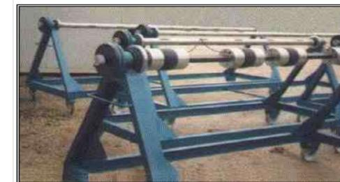
Mechano pneumatical or manual reel riser
